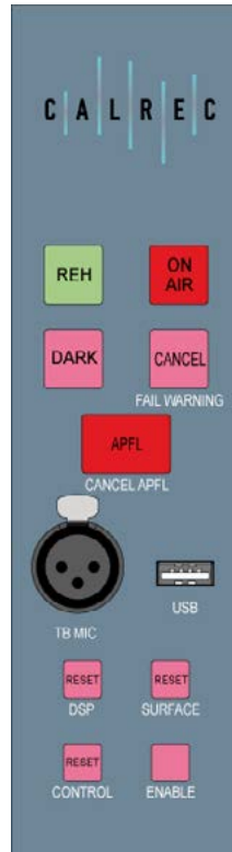
FIG 10 - BROADCAST FACILITIES PANEL
