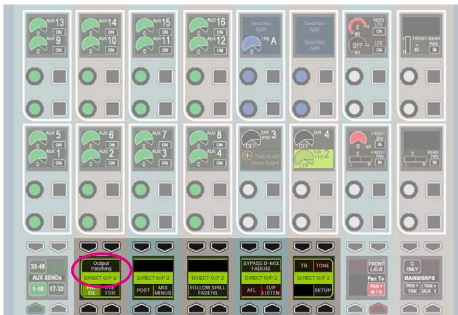
FIG 3 - ADDITIONAL CONTROLS FOR EACH DIRECT OUTPUT
