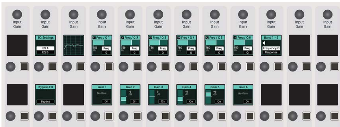
FIGURE 1 - CONTROL CELLS—ACCESS MODE—EQ
