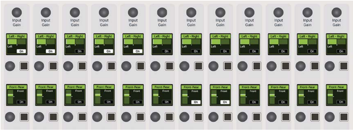
FIGURE 2 - CONTROL CELLS IN PAN CONTROL MODE
